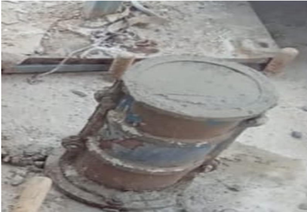
FIG 4.5 Casting of cylinders by using groundnut shell powder
