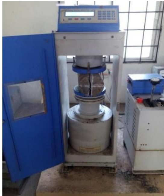
Fig 5.4 Testing on cylinder
