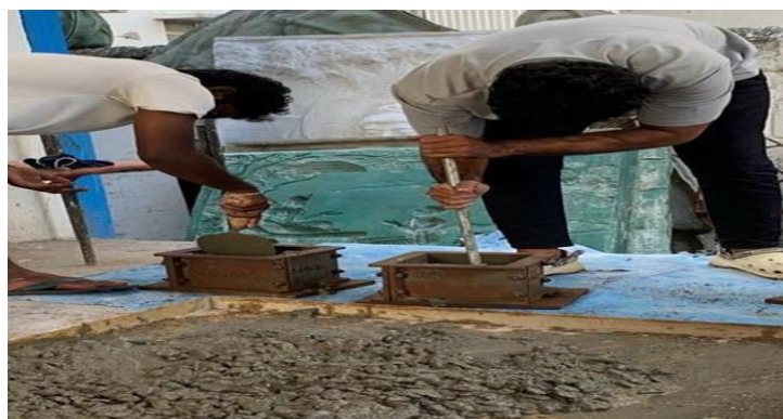
FIG 4.7 CASTING OF CUBE
