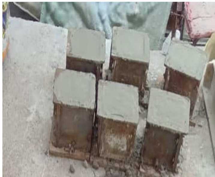
Fig 4.4 Casting of cubes by using groundnut shell powder
