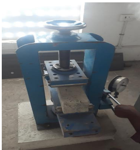
Fig 5.6 Testing of flexural strength of beam
