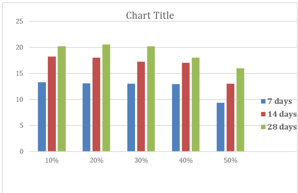
Fig 5.3 Compression strength of cube
