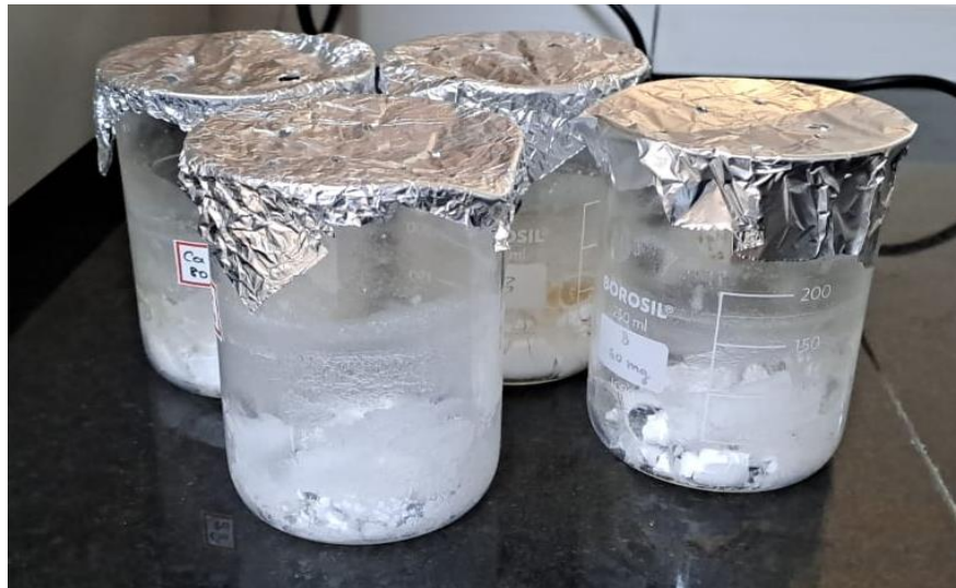
Fig.5.1: Diopside solution kept in hot air oven
