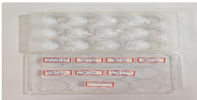
Fig.4.9: Biodegradation test of pellets in SBF
