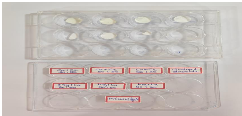
Fig.4.10: Pellets immersed in SBF for 30 days
