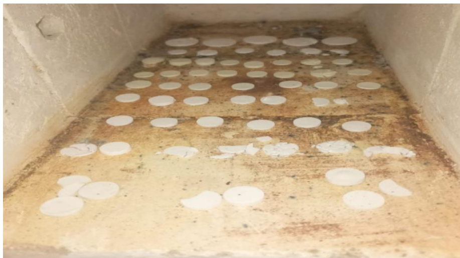
Fig.5.2: Pelletizing the diopside powder and sintering
