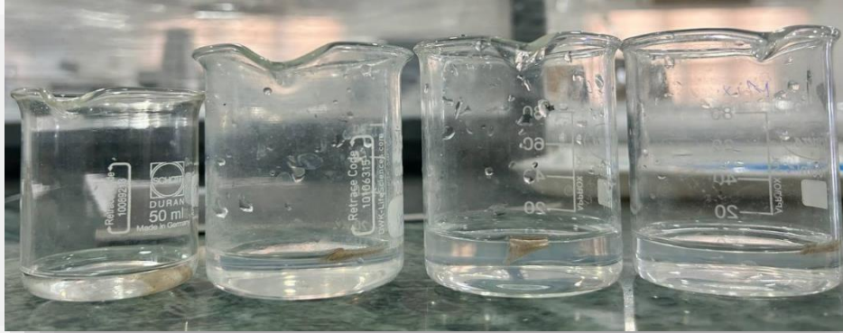
Fig 4.14 swelling test between each individual cellulose-based bioplastic with mixed three different source cellulose-based bioplastic
