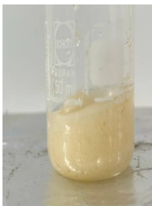
Fig 4.13 Representation of cellulose solution blended with polymer and chitosan
