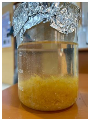
Fig 4.9 Representation of acid treatment for coconut coir
