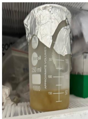
Fig 4.11 Representation of cellulose dissolution process with UREA/NaOH at -20°C
