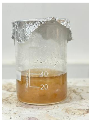
Fig 4.12 Representation of cellulose dissolution process with DMSO
