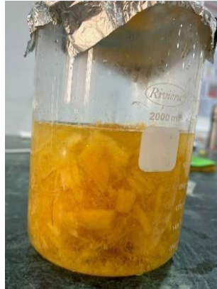
Fig 4.5 Representation of bleaching process for sugarcane bagasse
