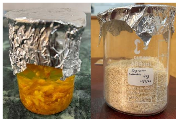
Fig 4.6 Representation of acid treatment and drying process for sugarcane bagasse
