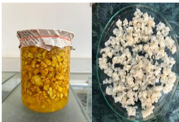
Fig 4.3 Representation of acid treatment and drying process for corn cob
