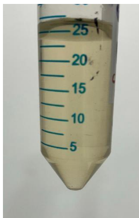
Fig 5.8 Representation of dissolved cellulose in zinc chloride.
