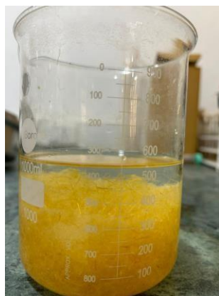
Fig 4.8 Representation of bleaching process for coconut coir
