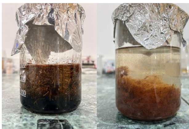
Fig 4.7 Representation of pre alkaline and alkaline process for coconut coir
