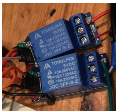
Fig:4.14: Relay switch for ESP 32
