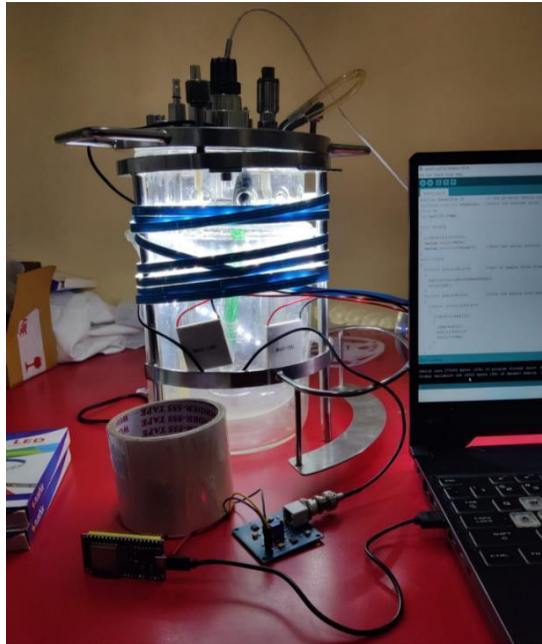
Fig:5.4: Optical sensor testing in photo bioreactor
