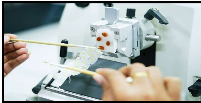
Fig : 1.7 Section cutting
