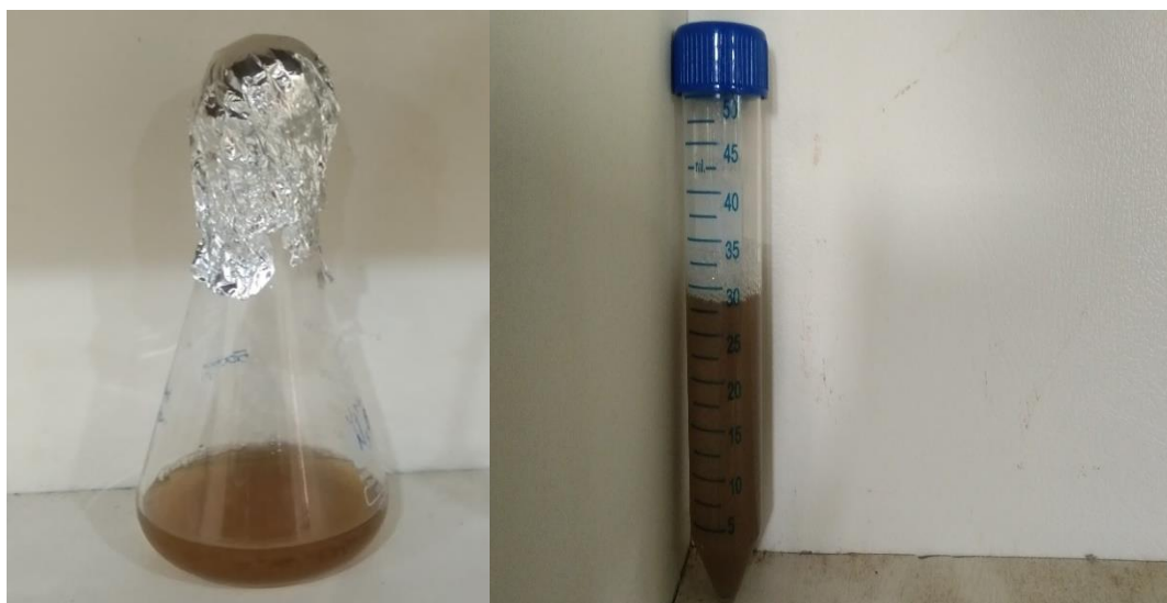
FIGURE: 5.9: The nanocomposite solution before and after autoclave for 5hrs
