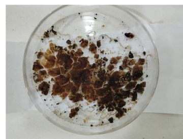
● Silica aerogel After drying in hot air oven for 6 hrs at 90°C
