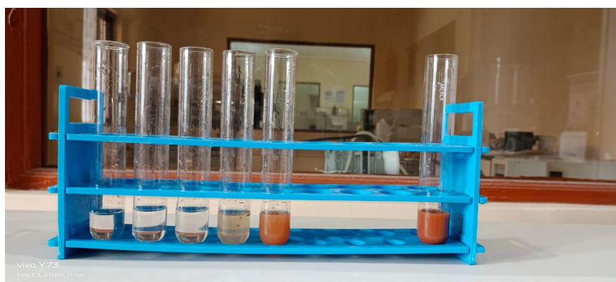
Fig:4.3: Serial dilution of soil samples
