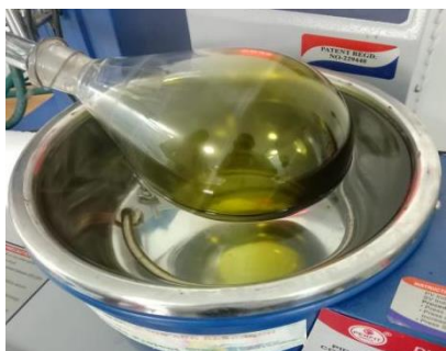
Fig 4.5: Subjecting the extracts in rotary evaporator.
