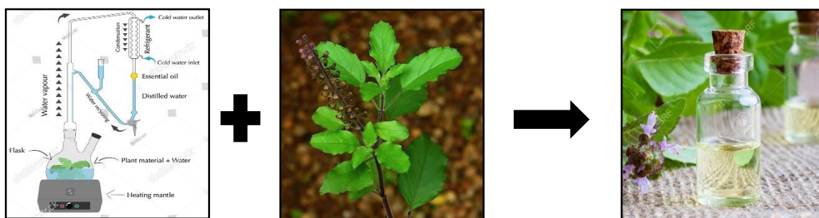
Fig 4.1: Hydro distillation of Ocimum sanctum leaves to obtain Eugenol
