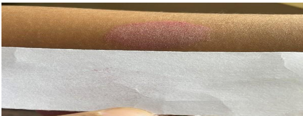
FIG 5.5 TRANSFER RESISTANCE TEST
