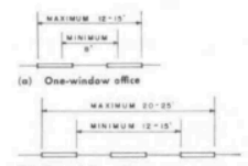
Fig. 11 Private office widths using a module of 4 to 5 ft.
