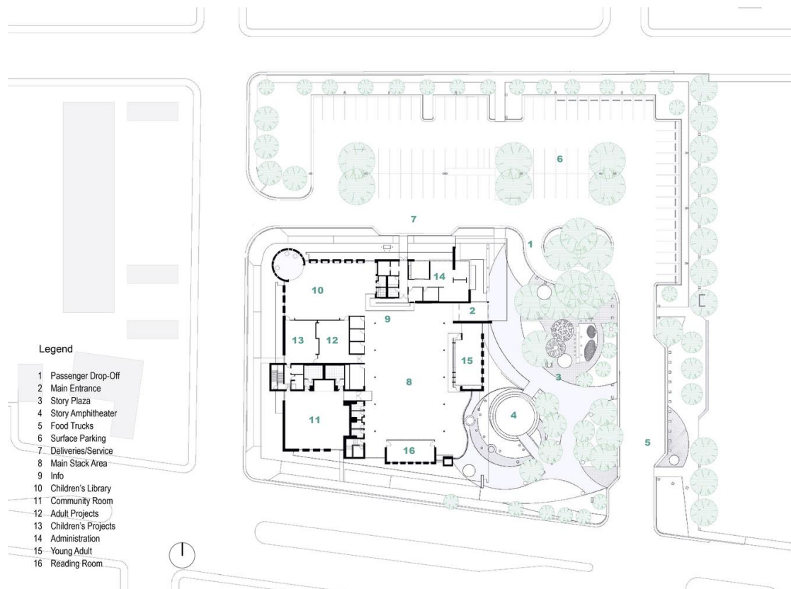
Figure 3.1: CABQ LIBRARY SPACES GROUND FLOOR
