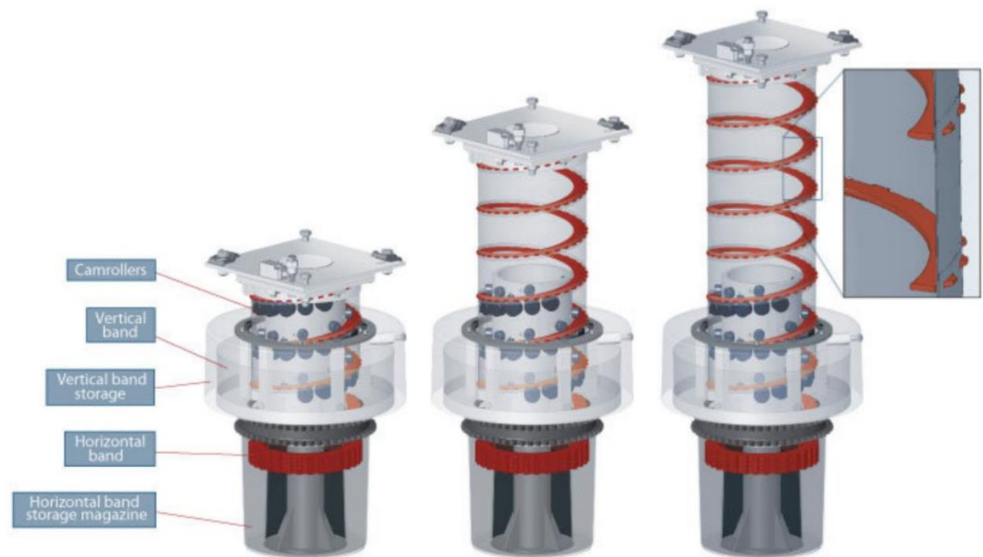
Fig 3.2: Components of spiralift
