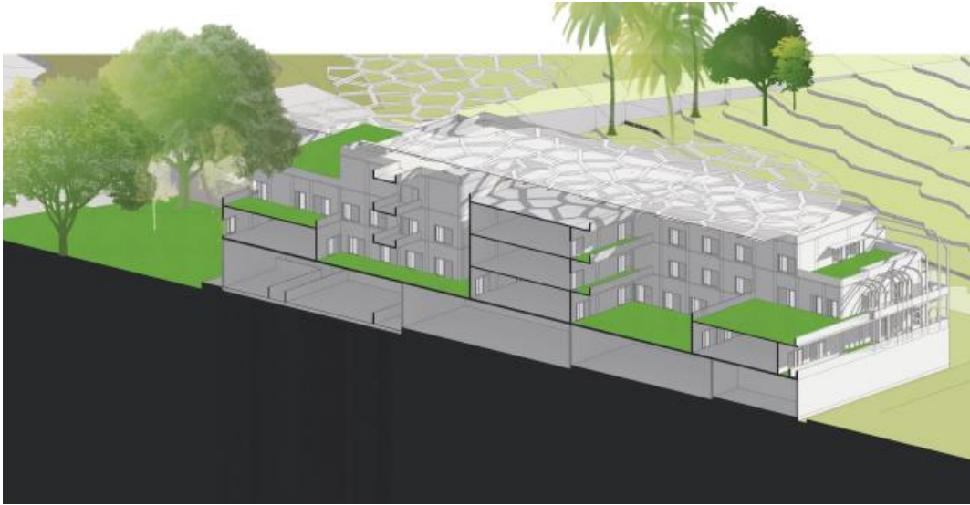
Fig 5.10: Isometric Section showing Green Roofs
