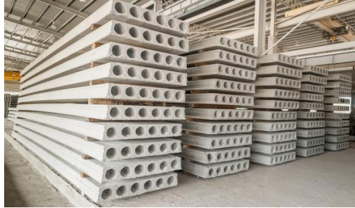
Figure 6.7 Hallow core concrete slab
