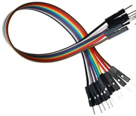
Fig:2.9: Jumper Wires
