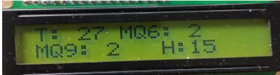
Fig 7.1 Temperature, MQ6, MQ9 and Humidity sensor Initial Data
