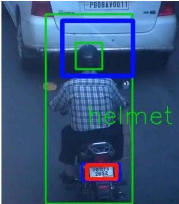
Bounding Boxes using SSD Algorithm
