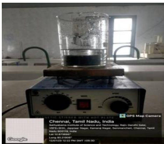
Fig.4.1: Stirring of rGO solution in waterbath
