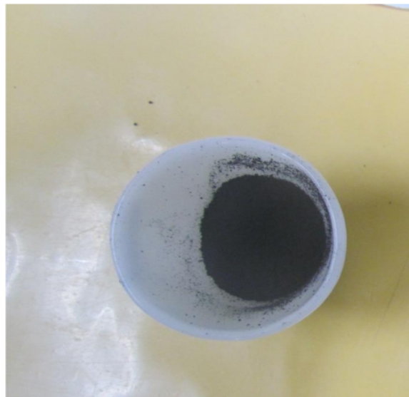
Fig: 5.3 : Soot content in scrubber tank (Initial)
