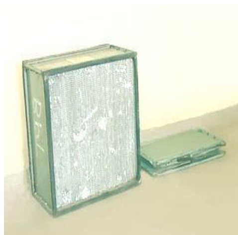
Fig: 2.2: HEPA filter before & after compaction, VRF ~ 10
