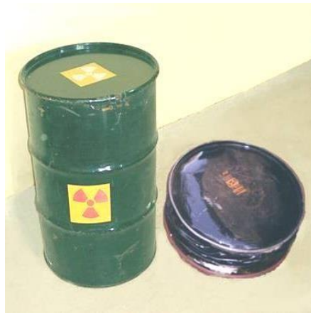
Fig: 2.1: Drum before & after compaction, VRF ~ 6
