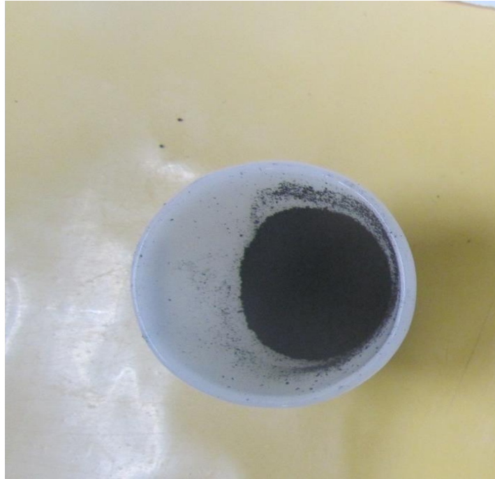
Fig: 5.3: Soot content in scrubber tank (Initial)
