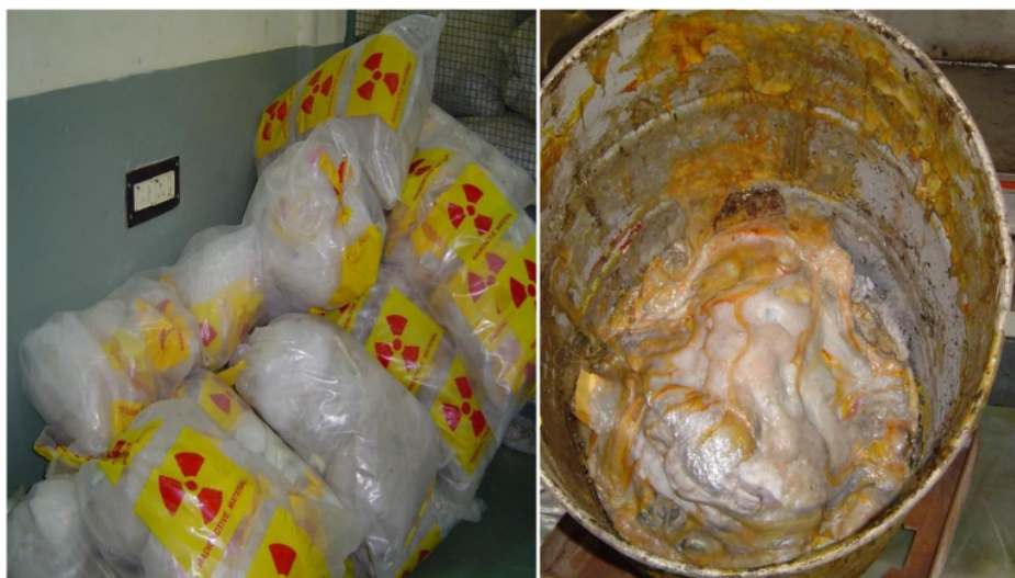
Fig: 2.5 : Polythene waste before and after MDU operation
