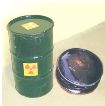
Fig: 2.1 : Drum before & after compaction, VRF ~ 6
