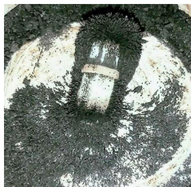
Figure 4.9: Attraction of Magnetic Chitosan to external magnet
