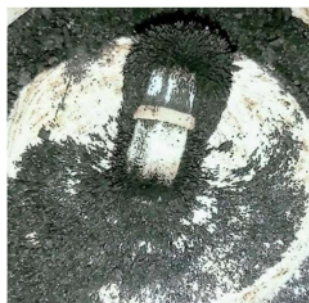
Figure 4.9 : Attraction of CS-MNP to magnet
