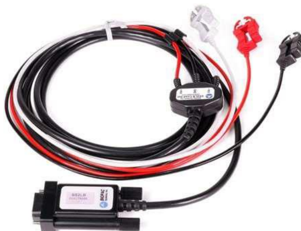
Fig 4.5 SS2LB – Lead selection circuit
