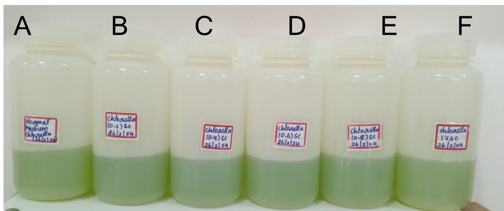
Figure 5.2.1 Control (A), sample (B) 0.20% NaHCO 3 , sample (C) 0.40% NaHCO 3 Sample (D) 0.60% NaHCO 3 , Sample (E) 0.80% NaHCO 3 , Sample (F) 1.00% NaHCO 3 . PICOCHLORUM , CHLORELLA
