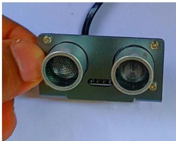
Fig 4.7 Ultra sonic sensor
