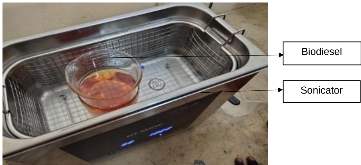
Fig: 4.6 Sonicator for mixing alumina nanoparticles with biodiesel blends
