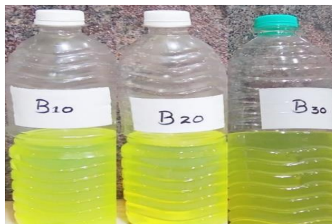
Fig: 4.5 B10, B20 and B30 blends of biodiesel
