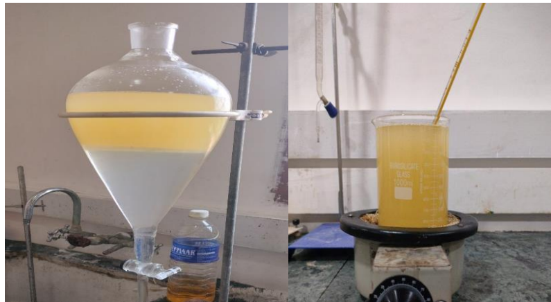
Fig: 4.4 Washing and drying of biodiesel
