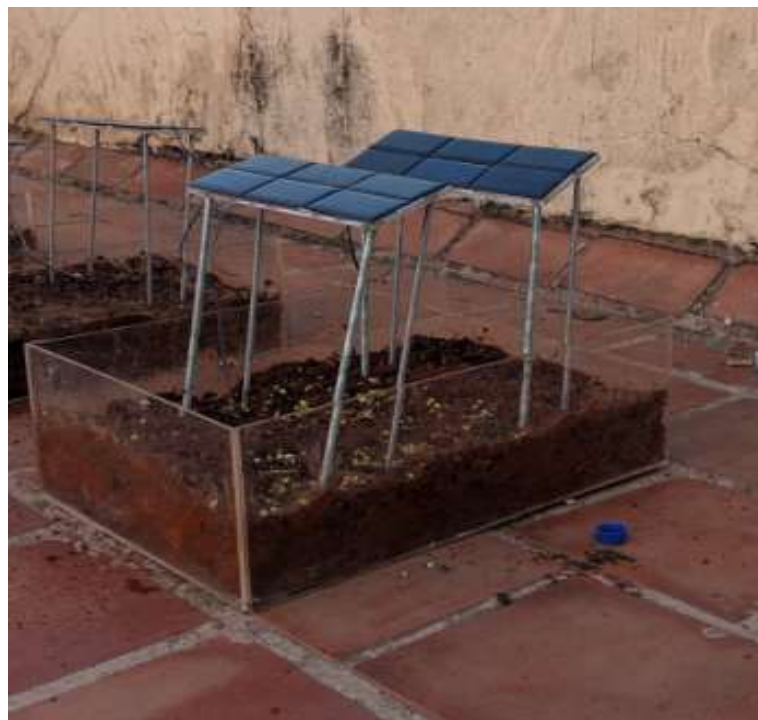
Fig :5.6: 25° Tilted Solar Panels
