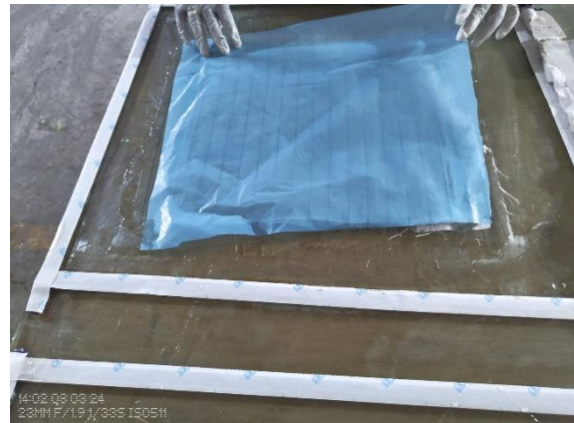
Fig 4.8 Vacuum Bagging Assembly
