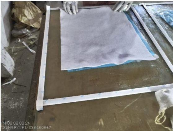
Fig 4.7 Vacuum Bagging Assembly
