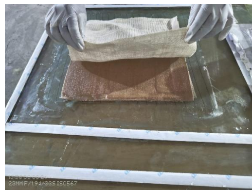
Fig 4.4 Layup of Fiber Reinforcement
