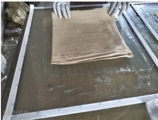
Fig 4.3 Layup of Fiber Reinforcements
