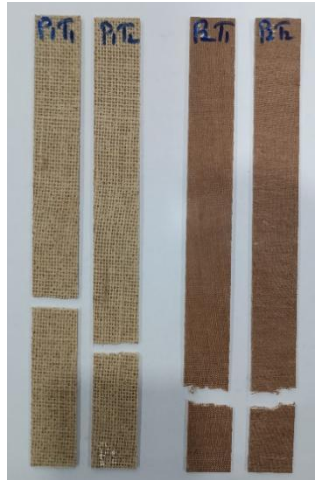
Fig 5.12 Tensile Specimen (After Test)
