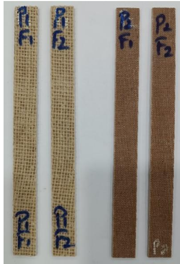
Fig 5.7: Flexural Specimen (Before Test)
