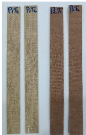
Fig 5.11 Tensile Specimen (Before Test)
