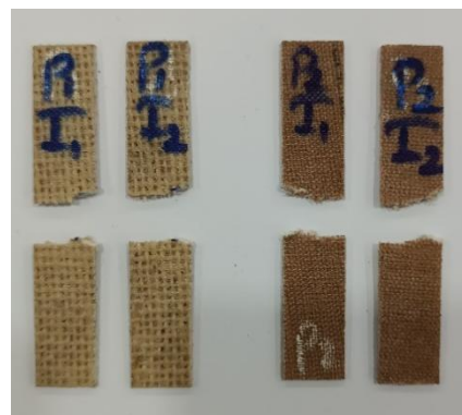
Fig 5.4 Izod Specimen (After Test)
