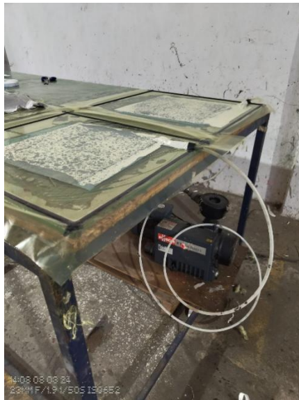
Fig 4.9 Sealing and Evacuation
