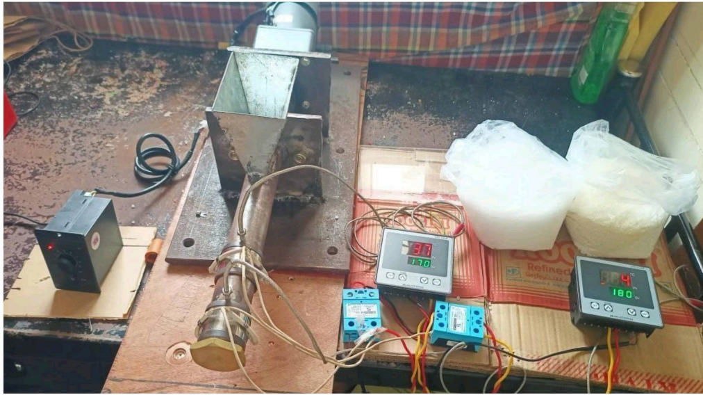
Figure 4.9: Heaters with Thermocouple Attachment to Barrel
