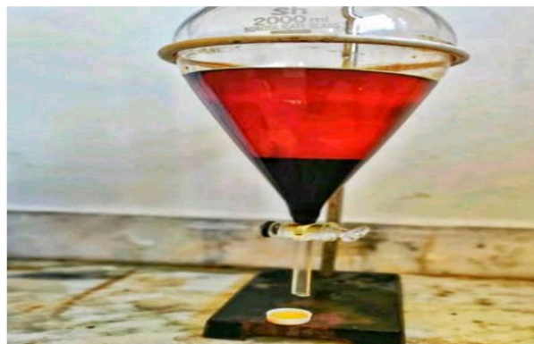
Fig: 4.5: Extraction of bio-diesel from waste cooking oil
