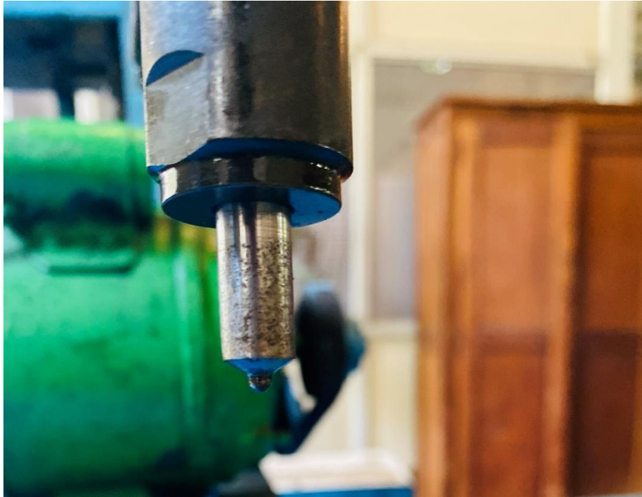
Tip of 2-hole nozzle (fuel injector)
