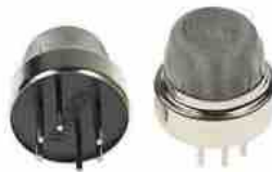
Fig:3.8: Gas Sensor
