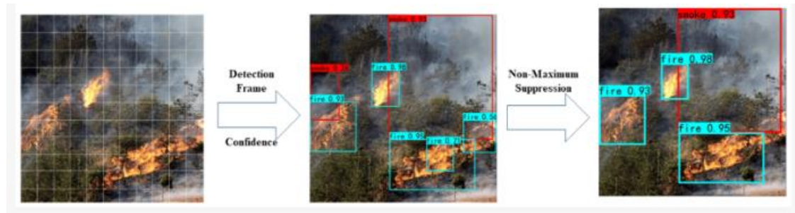
Fig 5.2 Fire Detection using Image Processing
