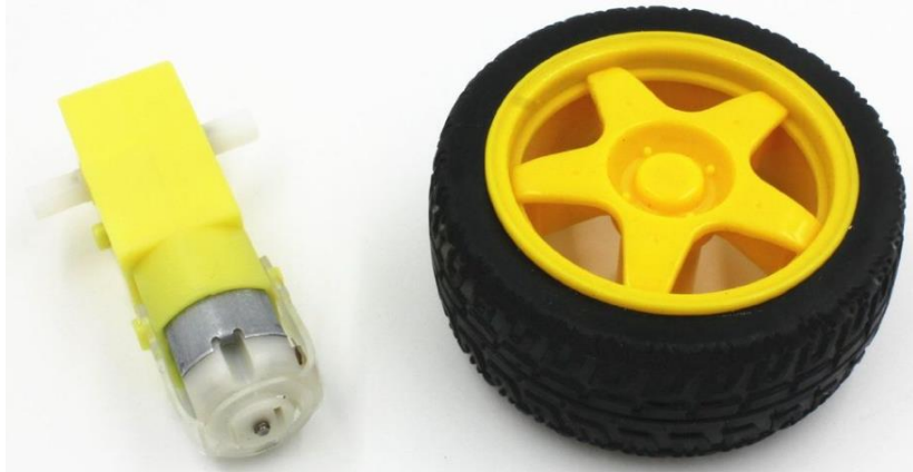
Fig.3.6: DC Gear Motor
