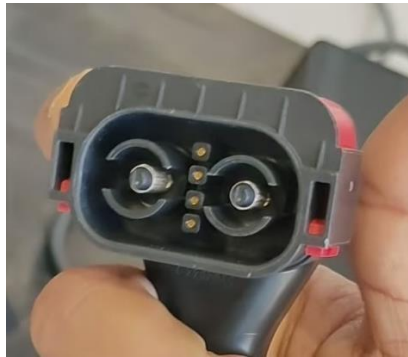
Fig. 4.2. Charging Pin of Ampere Primus
