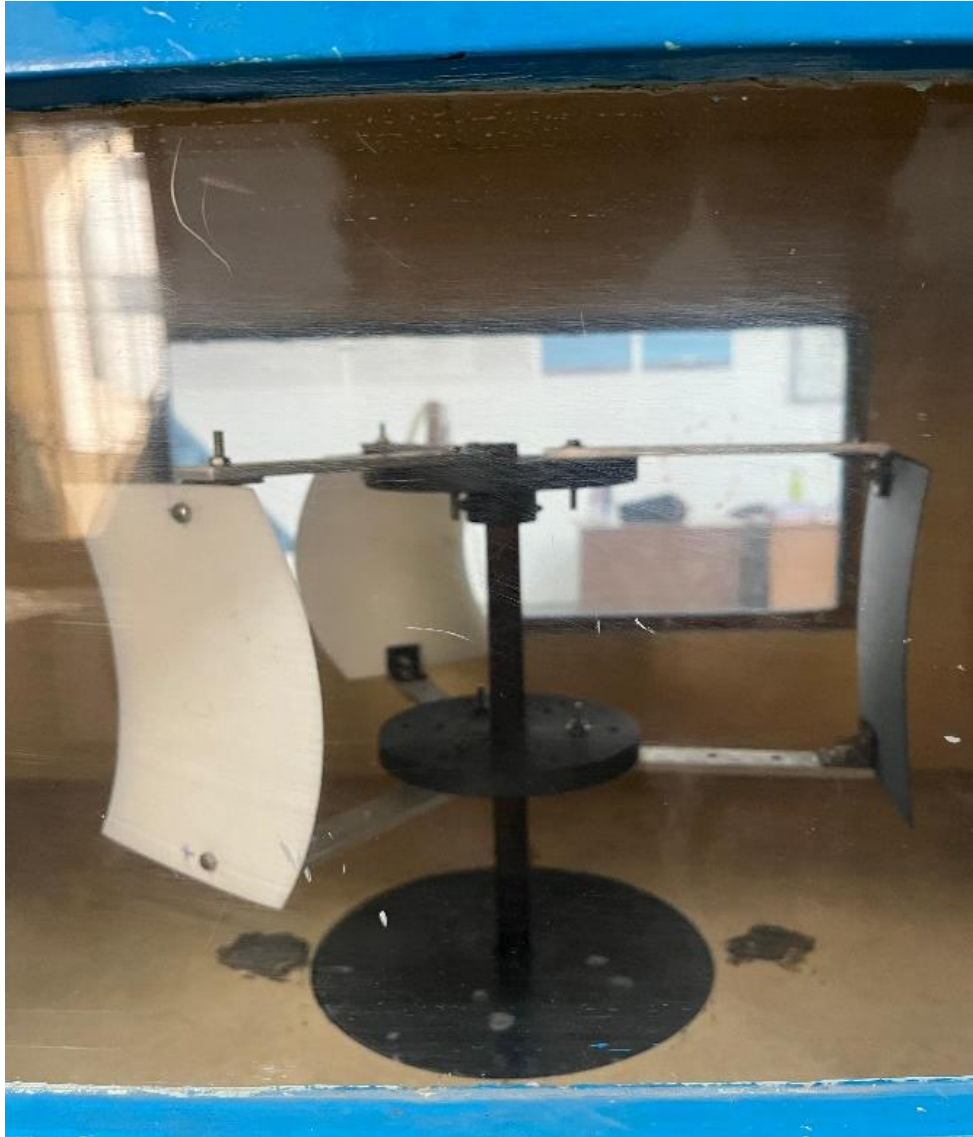
Fig:5.8 : Wind turbine in test section
