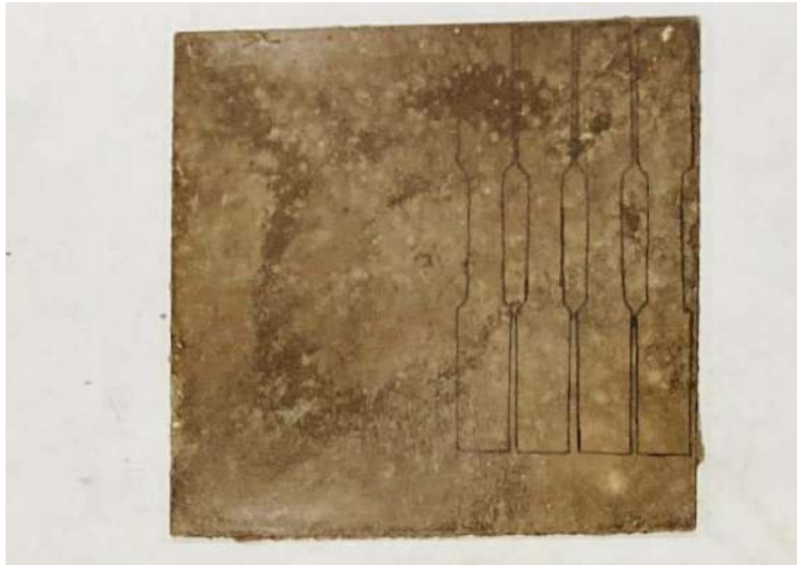
Fig 4.7 Untreated banana fiber + PLA composite
