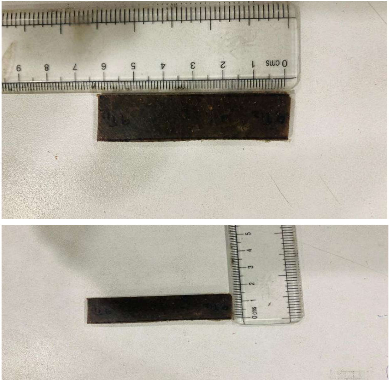
Fig 4.11 Impact samples with measurements
