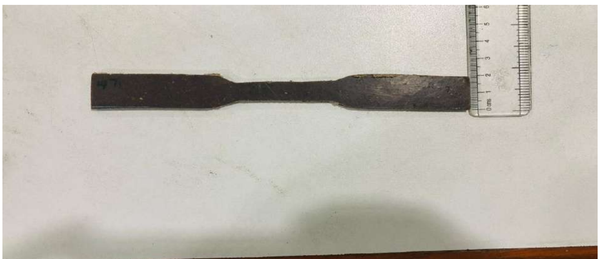
Fig 4.9 Tensile sample and measurements
