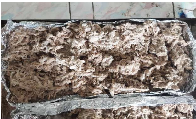
Fig 4.3 Untreated fiber dried with hot air oven
