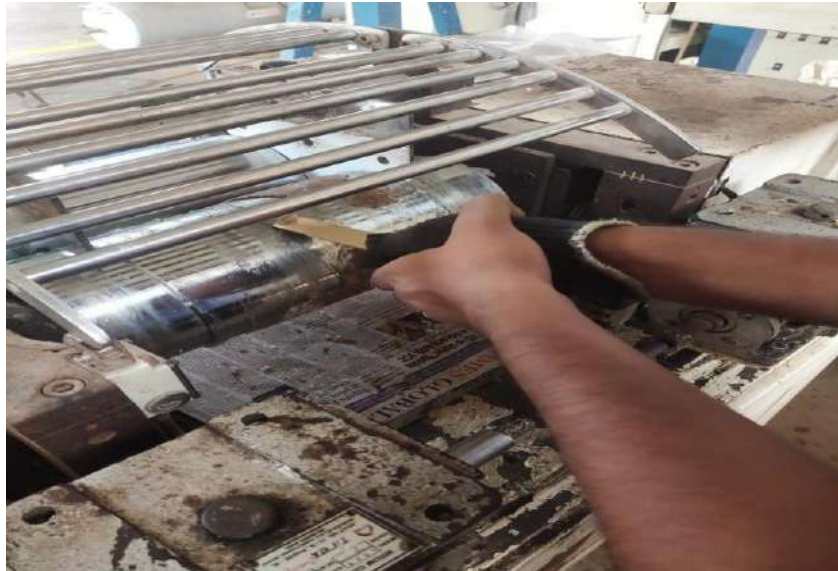
Fig 4.5 Preparation of PLA and Banana fiber sheets using to roller machine
