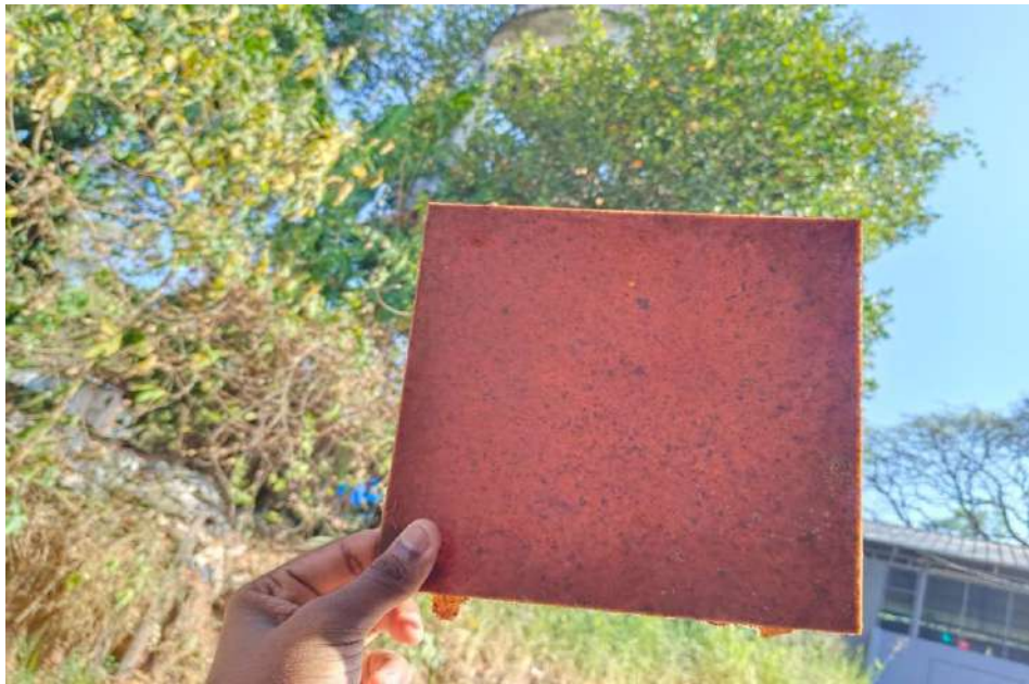
Banana fiber composite plate
