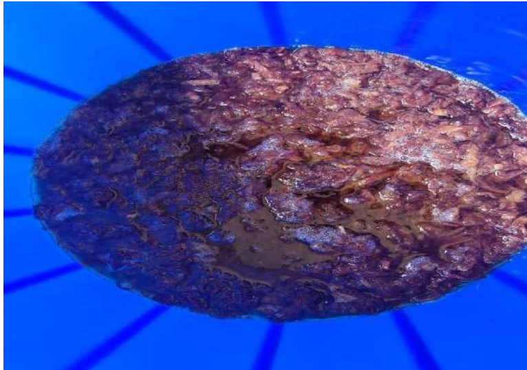
Fig 4.2 Fiber treated with NaOH chemical
