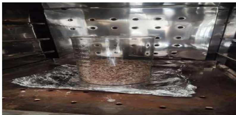
Fig 4.4 Removing excess moisture using hot chamber
