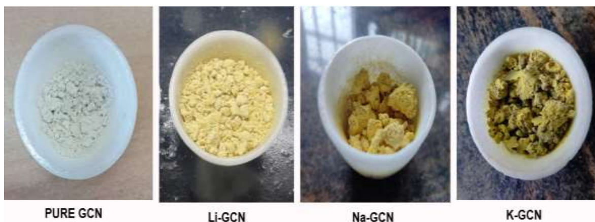
Fig:5.1: Synthesised Pure g-C 3 N 4 And Doped g-C 3 N 4
