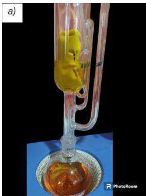
Fig 5.1: a) Soxhlet extraction of turmeric b) Separation using separating funnel
