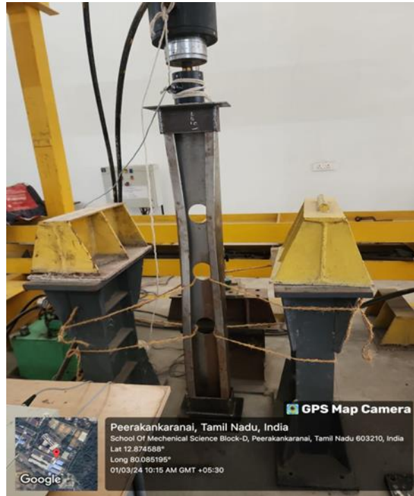
Figure. 4.9: Unstiffened G-section column with three opening
