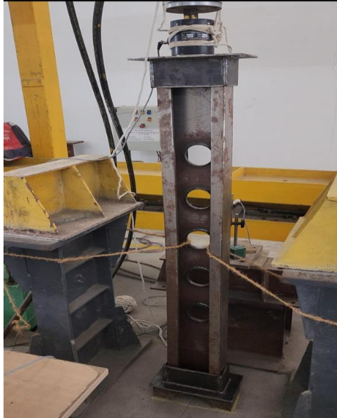
Figure.4.15 Stiffened G-section column with five opening
