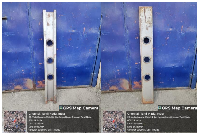
Figure.4.5: Fabricated stiffened G-section column with three openings
