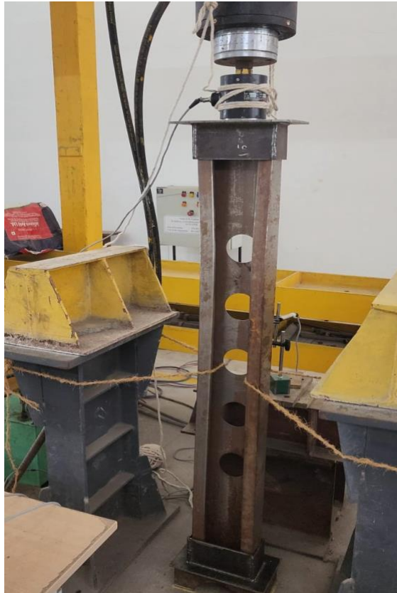
Figure.4.13: Unstiffened G-section column with five opening
