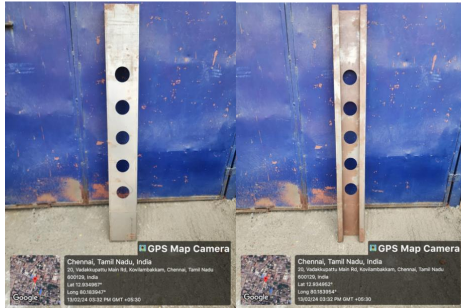
Figure.4.6: Fabricated unstiffened G-section column with five openings
