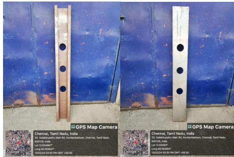
Figure.4.4: Fabricated unstiffened G-section column with three openings
