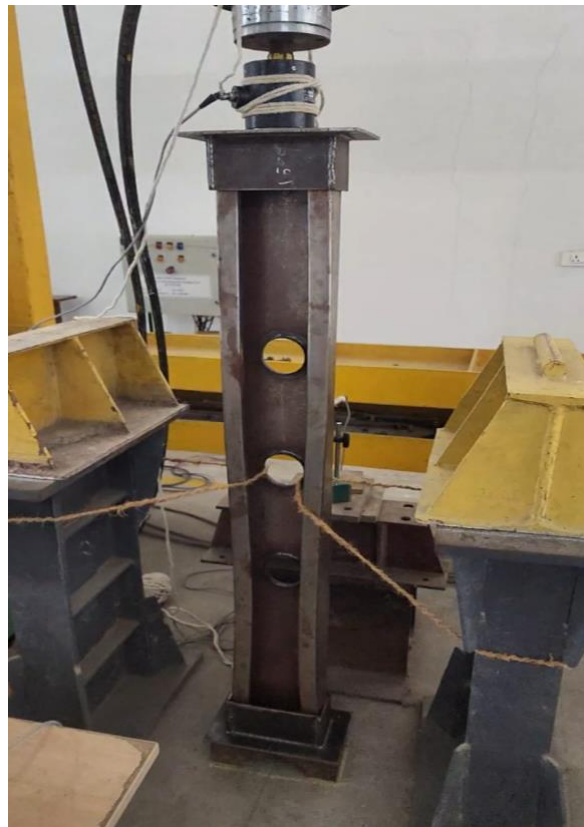
Figure. 4.11: Stiffened G-section column with three opening
