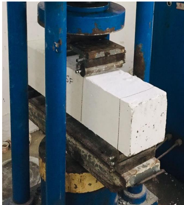
Figure 4.6 Flexural strength testing
