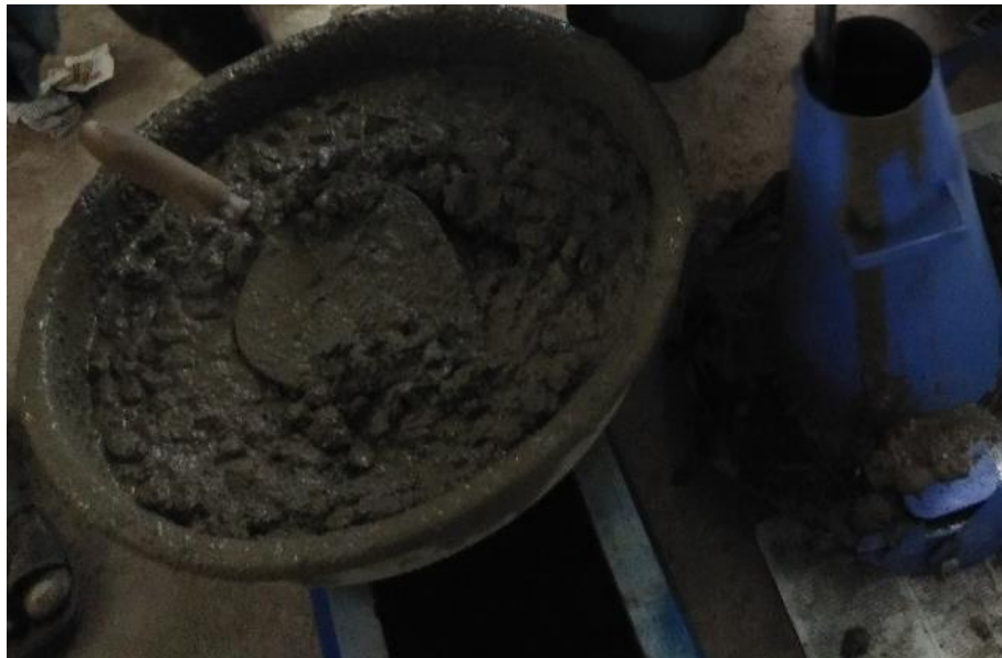
Figure 3.3 Slump cone test
