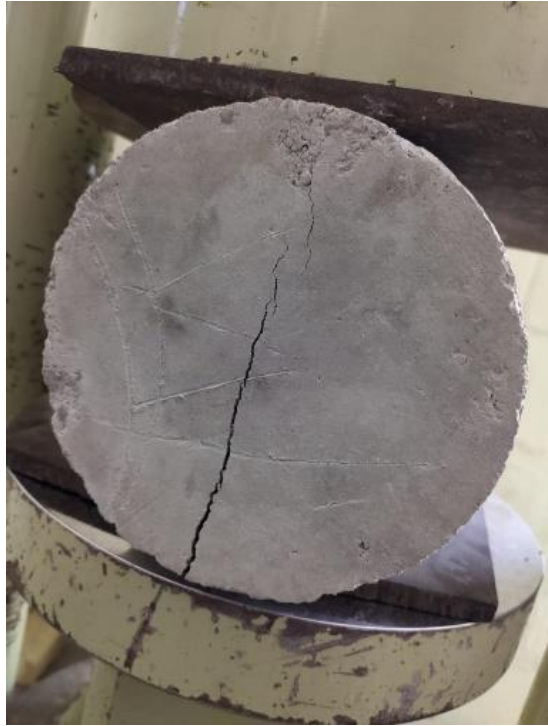
Figure 4.4 Split tensile strength testing
