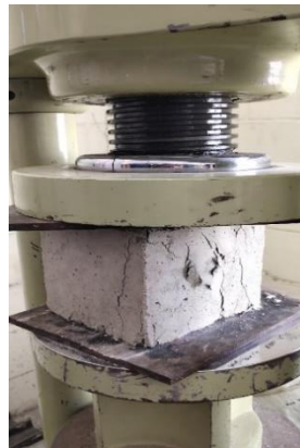
Figure 4.2 Compressive strength testing
