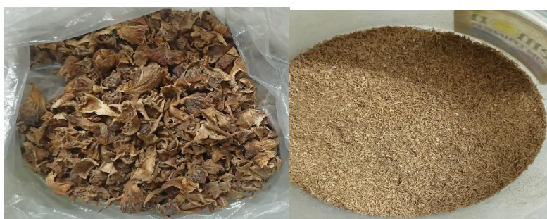
Fig 4.1: (a) Dried pineapple peel; (b) Powdered pineapple peel.
