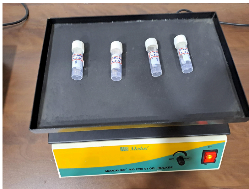
Fig 4.7 Elution of metal samples using a gel rock and shaker
