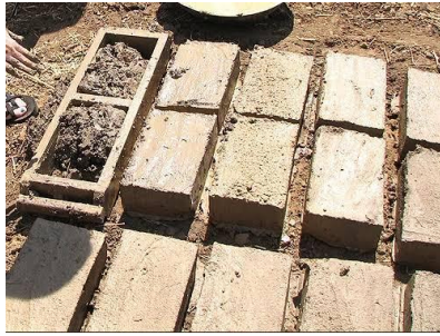
Fig 4.9 Molding of bio-composite brick
