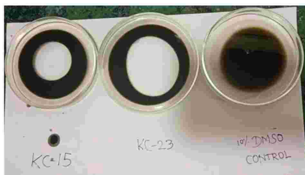
Fig:5.16 Bacterial strain KC15, KC23 shows biosurfactant production
