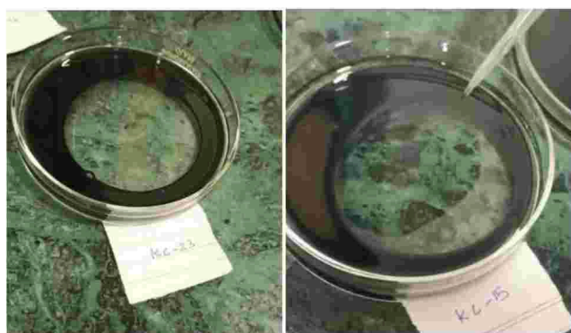
Fig: 5.2. oil displacement assay for KC-15 and KC-23 samples
