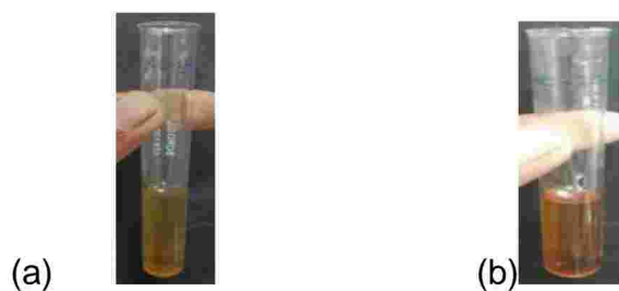
Fig:5.5 KC15, KC23 reacts to phenol sulfuric acid test
