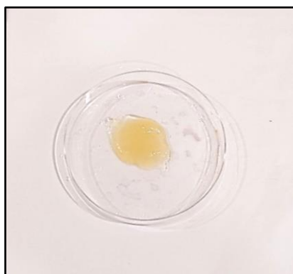
Chitosan hydrogel prepared using cross linker glutaraldehyde
