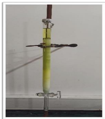
Fig: 5.4. Column Chromatography (Gracilaria)
