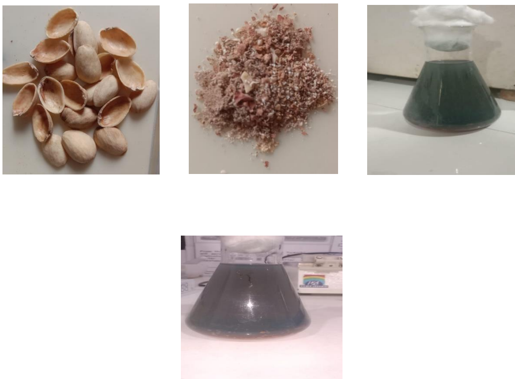
Fig 5.1: Synthesis of copper nanoparticle using Pistachio shells
