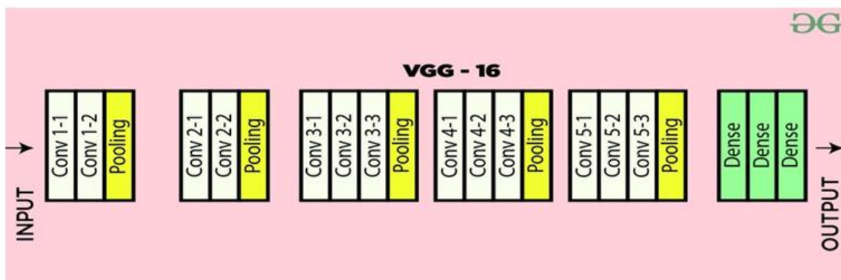
Figure 9 - VGG16 layered architecture
