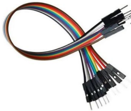
Fig:2.9: Jumper Wires
