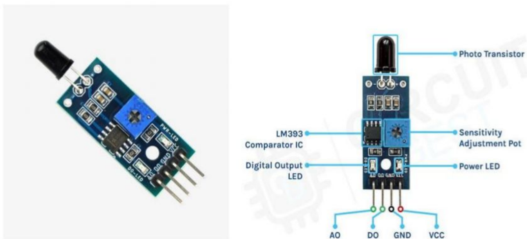
FIG 2.2 FIRE SENSOR
